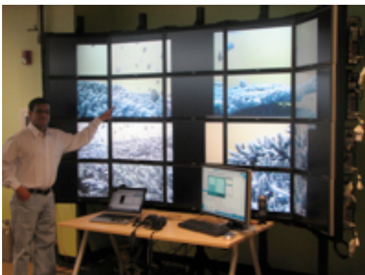
Figure 2: Tiled Display Wall (TDW) at Calit2 (UCSD) showing data from underwater video cameras in Kenting (Taiwan) in real time using DataTurbine streaming data middleware.
