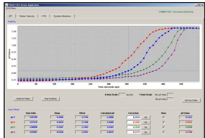
Fig. 7: Step response of four pH sensors to injection of  $CO_2$  enriched seawater. Time proceeds from right to left in this chart (like a strip chart recorder). Note the time lag between the four sensors, representing their physical placement in the chamber and the movement of water past each sensor.
